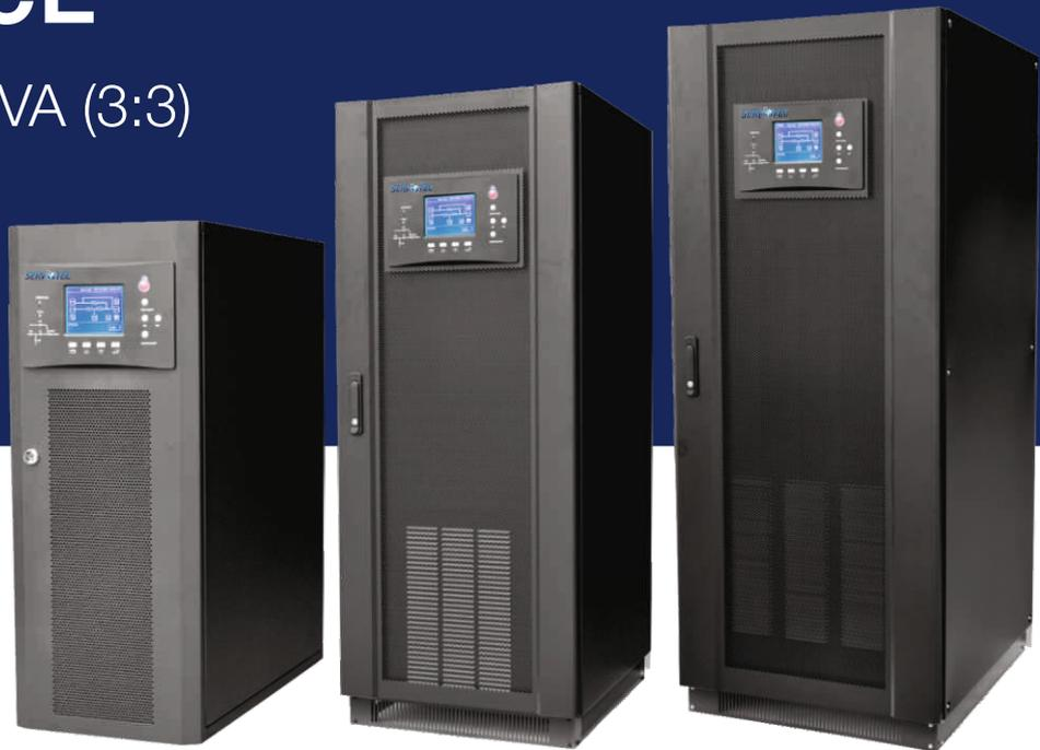
Flurance series UPS is a intelligent 3 phase in 3 phase out uninterruptible power supply, it adopts double transform high frequency PWM and high performance digital control technique (DSP), with perfect protection, super network management function, reasonable man-machine interface and a series of precision design, meets all high reliability requirements of uninterruptible power supply and integrates reliable, safety, maintainability characteristics of a new generation low frequency UPS.
