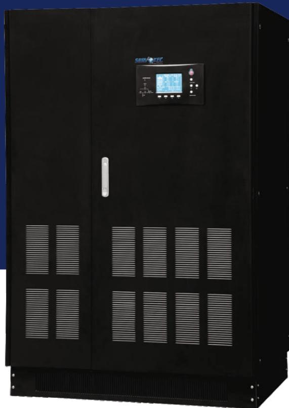
Flurance series UPS 80 ~ 500 kVA provide maximum protection and power quality for mission critical loads, including data centers, industrial processes, telecommunications, security and electro-medical systems. It is an on-line double conversion UPS with IGBT-based 3-level PWM rectifier technology, featured with high input power factor ( $> 0.99$ ), low THDi, high efficiency (max.  $\geq 94\%$ ) and built-in output isolation transformer.
